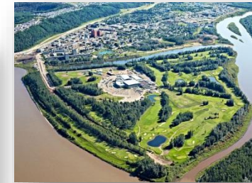
MacDonald Island, AB, Canada Integrated Water Reuse and Heat Recovery system utilizing treated wastewater effluent for irrigation and flush water while also recovering the effluent heat for pool heating within the rec center.
